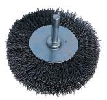
Suitable for use in power drills. Most useful for hard to reach areas and grooves. 6mm shank. Specifications: 9584.0550: (Dia)50mm x (W)25mm. Max rpm: 15,000. 9584.0560: (Dia)60mm x (W)25mm. Max rpm: 15,000. 9584.0570: (Dia)70mm x (W)25mm. Max rpm: 15,000. 9584.0580: (Dia)80mm x (W)25mm. Max rpm: 12,000.
