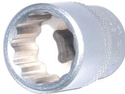
Ideal for assembly and servicing of small precision mechanisms associated with electrical, electronic, ignition and refrigeration work. All bi-hexagon unless stated. Double knurl feature gives a high grip which is essential for a quick tool change when your hands are greasy/oily. The 12 point bi-hexagon side drive design will give a higher torque than normal sockets.
