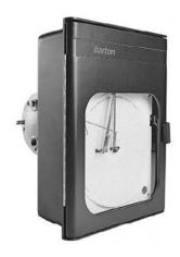
Barton Single Pen Temperature Recorder, Model 242E, Temperature Range: 0-100 DEG C, Mechanical Chart Drive: 24 HRs/7 Days
