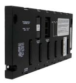
5-slot rack with an embedded CPU in base, 6K Bytes User Program. It's a 16-bit system belonging to the 90-30 series of PLCs with a processor speed of 10 MHz and a registry memory of 1 kilobyte. It comes with 160 Input / Output points with no Floating-point math.
