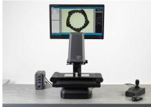
When quick throughput and user-friendliness are crucial, the TVM digital measuring microscope is an excellent option for a shop floor non-contact measurement system for 2D measurements of both turned and flat components. The motorized stage can measure larger components quickly and automatically.
