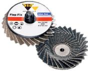
Siamet 2824 Active additives help with grinding properties, cotton backing breaks down to expose fresh grit. Fast, safe and easy disc change offered by Siafix system. Zirconia alumina grit flap cup with X-weight cloth/cotton backing. Used for dressing of mild and stainless steel weld seams and joints in hard to reach areas. Backing pad required.
