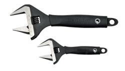
Drop forged chrome vanadium steel. Rubber comfort grip handle. Ideal for use in plumbing, installation and automotive applications. Ultra thin head designed for use in confined spaces. Graduated millimetre scale. More than 50% wider jaw compared to conventional adjustable wrenches. Conforms to: ISO 6787-1982, ASME B.107.8M-1996, BS 6333-1995, DIN3117-1988, JIS B4604-1976. Set contents: 1x 150mm and 1x 250mm.
