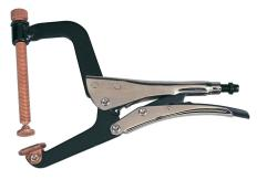
Fine spindle clamping adjustment enables accurate clamping. Swivel joint clamping points allow tapered surfaces to be securely clamped. Copper plated spindle and clamping points ensure weld splatter will not adhere.
