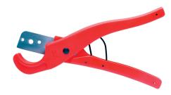
6 - 37mm cutting capacity. Spring opening. Lightweight moulded polypropylene body. Stainless steel blade. Guillotine action ensures a clean cut every time. Handle retaining hook for compact storage and blade safety. Reversible blade. Not suitable for cutting metal.
