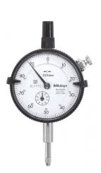
A Mitutoyo multi-revolution dial indicator suited to general measurement applications. The dual-reading scale aids measurement in both directions. Standard 0.01 mm graduation dial gauges having a bezel with an outside diameter of 57 mm. All types come with limit markers and a bezel clamp as standard.
