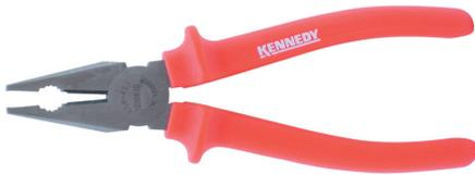
Universal type heavy-duty combination pliers with single cutter. Chrome vanadium steel with heavy-duty insulated handle with slip guard. Double polished head and joint. Serrated parallel jaws for gripping flat workpieces and a serrated curved jaw for gripping nuts, etc. Also with side cutter with induction hardened cutting edges.
