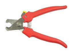
For cutting copper cable, plastic pipe, wooden dowels, rope cord and similar materials up to 10mm diameter. Precision ground and hardened stainless steel blades - 50~54HRC. Lightweight polypropylene handles with spring loaded action, easy reach thumb catch convenient for right and left hand users. Overall length: 165mm (6 1/2
