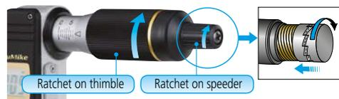
Ratchet-induced micro-vibrations along the spindle help ensure repeatable measurements.
