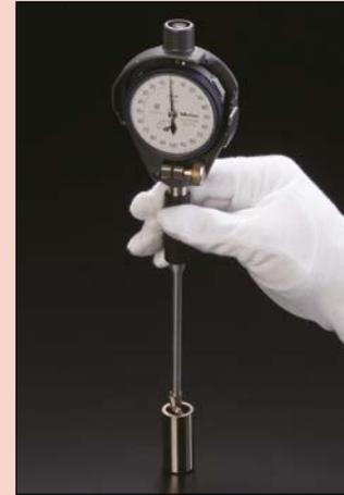
A heatshield prevents accuracy degradation due to hand heat during prolonged use.
