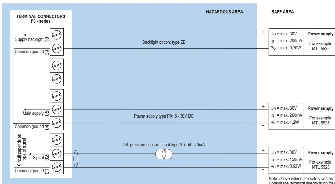
\* Sensor supply voltage for analog pressure sensor type A: not available in this example. Please note: type PX may be used in combination with the battery (type PC). PX will power the unit; the battery will be disabled automatically till power is disconnected.
