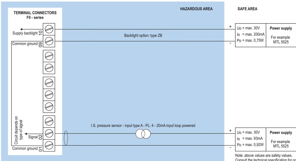
Sensor supply is not available: unit is input loop powered (type PL).
