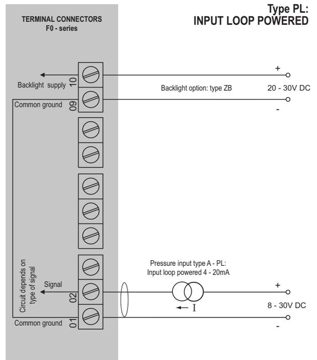
Sensor supply: sensor is externally powered.
