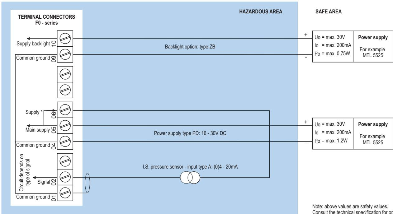
\* Sensor supply voltage for analog pressure sensor type A: Terminal 6: as input voltage terminal 5 (internally linked).
