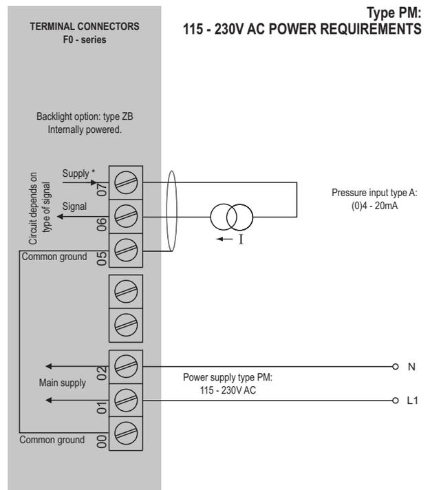
\* Sensor supply voltage: Terminal 7: 8.2 / 12 / 24V DC.
