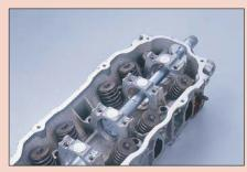
Rocker-arm bearing housing measurement using an extension
