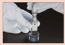
Measuring diameters down to 2 mm with the two-point
