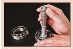
Ball-bearing inner-race inside diameter measurement.
