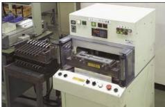
Air leak test equipment for coolant proof caliper.
