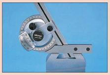
Measuring an internal dovetail slide angle.
