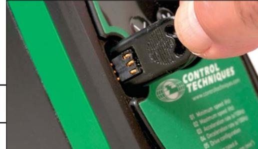
Makes multiple drive programming fast, and 100% reliable. Perfect for storing correct factory settings for maintenance records.
